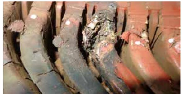
Failed winding due to molten copper dripping from rotor.
