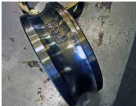
The difficult angle of the application lead to premature bearing failure.
