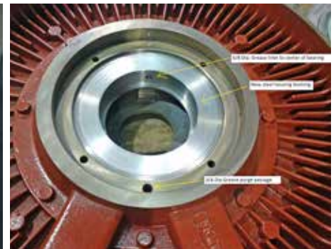
The modified grease inlets and outlets allow the redesigned bearings to properly re-lubricate.
