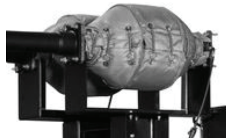
Typical 3-Way catalyst system
